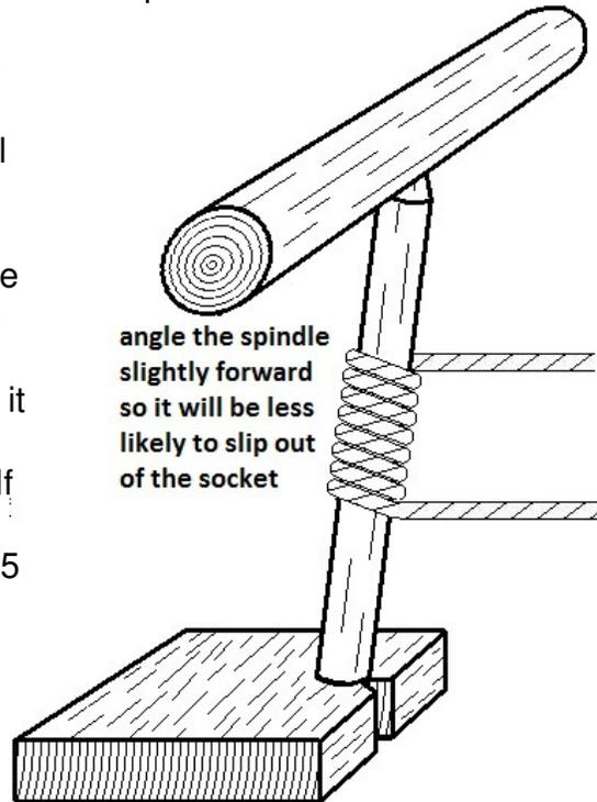
angle the spindle slightly forward so it will be less likely to slip out of the socket
