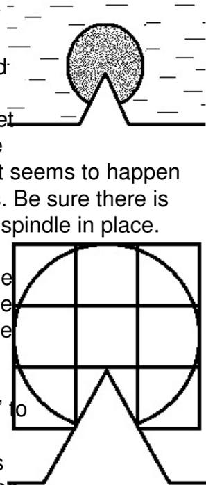
put it back into place, and start over. Try not to lose the dust that has already collected in the notch, as the notch must be full of dust before you can get fire. If the spindle appears to be starting to drill out of the notch, the pressure person can scoot forward on their seat a little to make the top of the spindle lean forward slightly, angling the base of the spindle back into the fire-board to help keep it in place. (See 'Trouble Shooting' later in this section).
