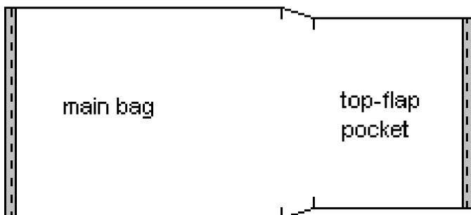
④ Fold under, and hem both ends. (From now on, the shading in the drawings represents the side of the material that will become the outside of the shoulder bag.)
